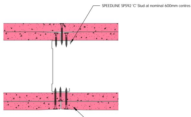
2 layers of 15mm British Gypsum Gyproc FireLine fixed with SPEEDLINE Drywall Screws at 300mm centres (200mm centres at external angles). Ref to table for fixing length.
